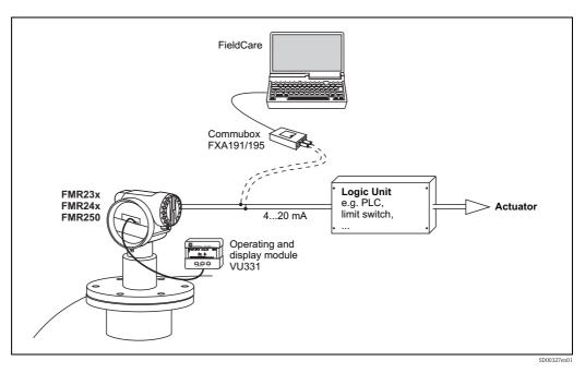
An analog signal (4 to 20 mA) in proportion to the level is generated in the transmitter. This is sent to a downstream logic unit (e.g. PLC, limit signal transmitter, etc.) where it is monitored to determine whether it is below or above a specified limit value.
