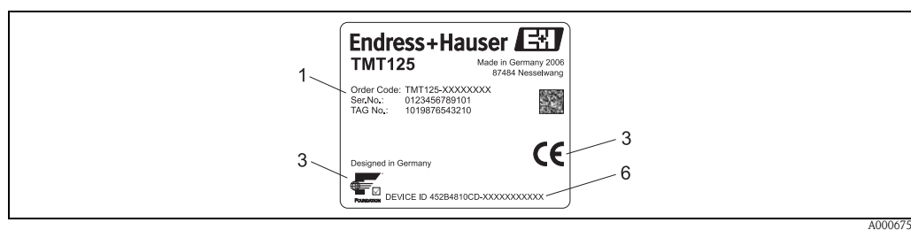
Fig. 2: Nameplate on the field housing (example)
