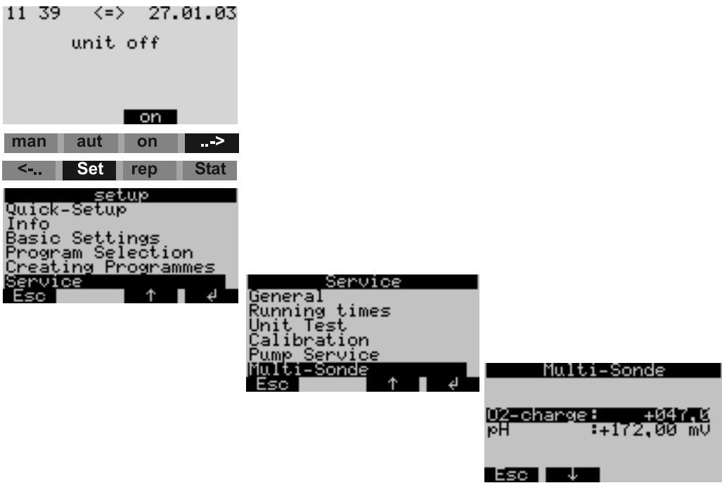
Fig. 33: Checking the oxygen measurement (sensor check system)
