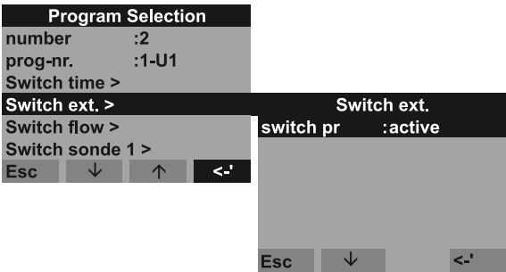
Fig. 45: Switching via external signal
