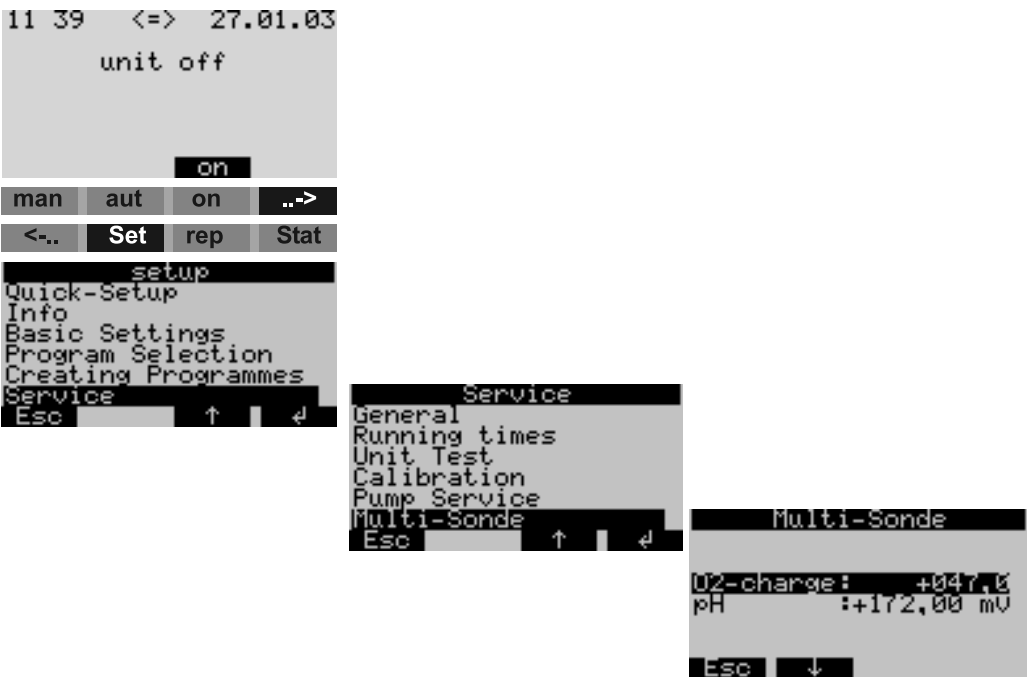
Fig. 29: Checking the pH measurement (sensor check system)
