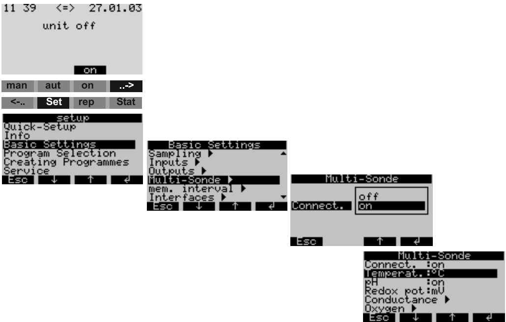
Fig. 34: Commissioning the multi-parameter probe (optional)
