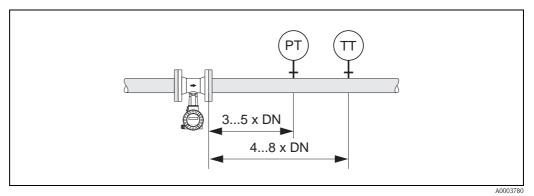
Fig. 9: Installation of pressure measuring point (PT) and temperature measuring point (TT)
