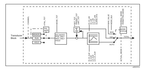
Fig. 35: Schematic illustration of the internal structure of a Totalizer function block
