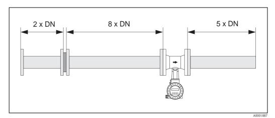
Fig. 10: Perforated plate flow conditioner
