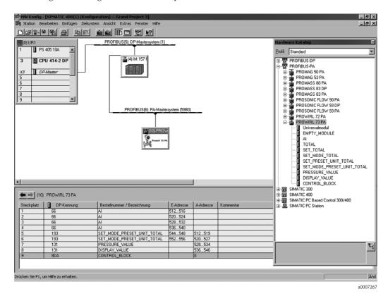
In this form of configuration, all the data blocks which are supported by the measuring device are activated.
