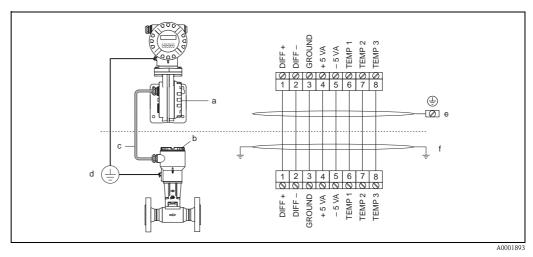
Fig. 15: Connecting the remote version
