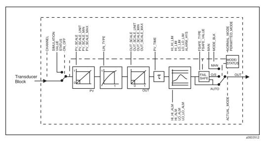
Fig. 33: Schematic illustration of the internal structure of an Analog Input function block
