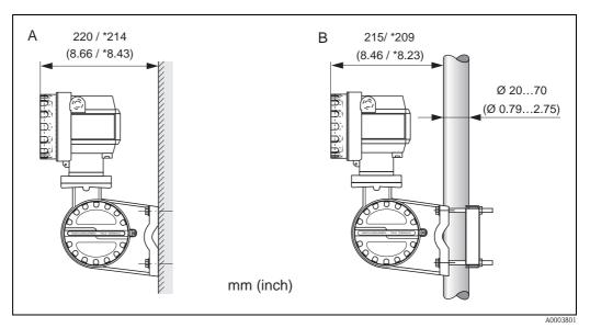
Fig. 14: Mounting the transmitter (remote version)
