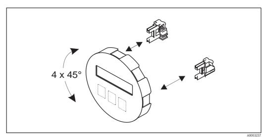
Fig. 13: Rotating the local display
