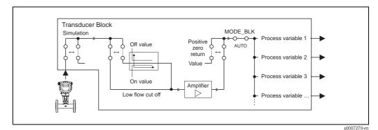
Fig. 32: Schematic illustration of the internal structure of the Transducer Block.
