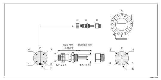
Fig. 19: Connectors for connecting to the PROFIBUS PA
