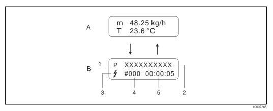
Fig. 23:  $A = Process \ variable \ display; \ B = information \ on \ the \ error \ message$
