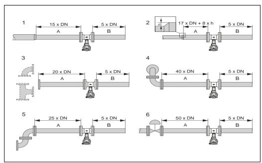
Fig. 8: Minimum inlet and outlet runs with various flow obstructions
