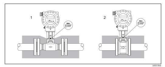
Fig. 7:  $1 = Flanged \ version, \ 2 = Wafer \ version$
