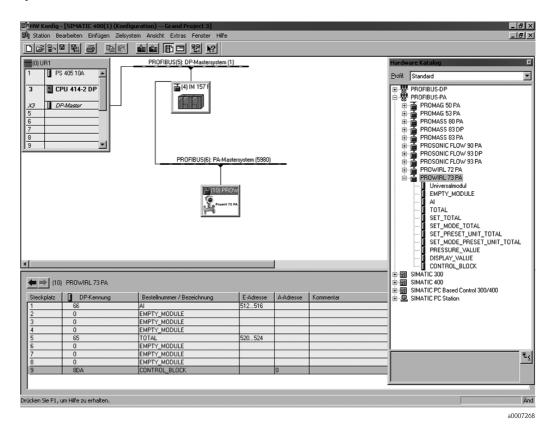
With this configuration, the Analog Input function block, the totalizer value TOTAL and the cyclic control of device functions CONTROL\_BLOCK are activated. The totalizer is configured "without configuration". In this example, it only returns the totalizer value and cannot be controlled. It is not possible to reset or stop the totalizer.
