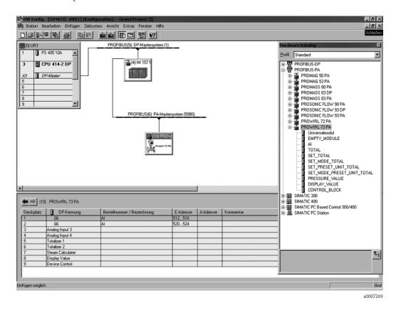
Analog Input function block 1 and 2 are transmitted with this configuration. If no further measured variables are required, the placeholders do not need to be used.
