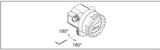
Fig. 12: Rotating the transmitter housing
