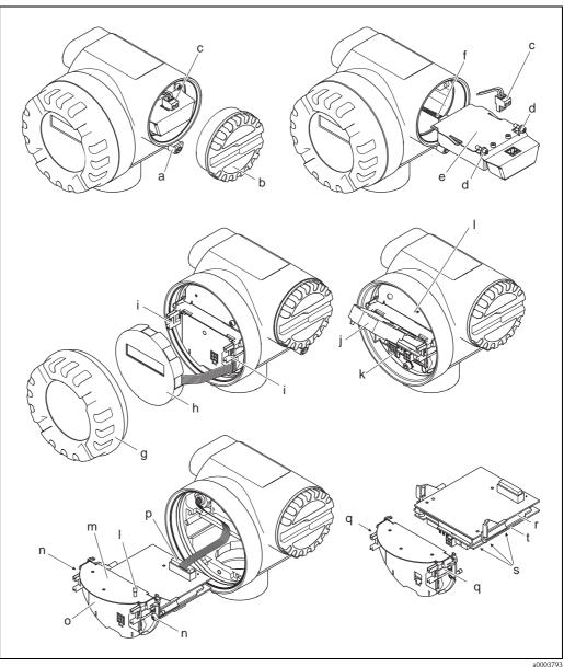
Installing and removing electronics boards, Ex d/XP version Fig. 30:
