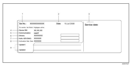
Fig. 3: Service nameplate specifications for transmitter (example)
