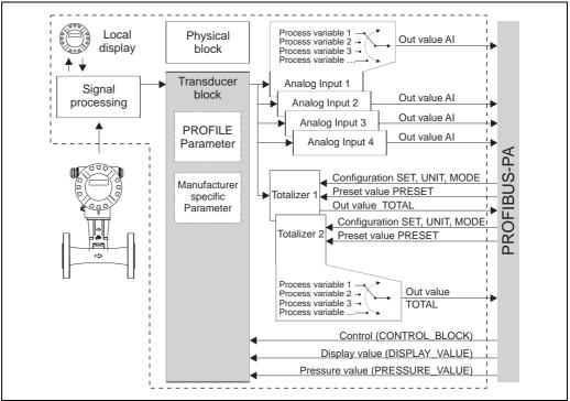
Fig. 27: Block model for Prowirl 73 PROFIBUS PA Profile 3.0
