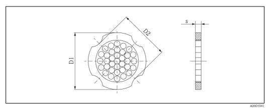
D1: The flow conditioner is fitted at the outer diameter between the bolts.
