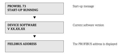
Normal measuring mode commences as soon as startup completes. Various measured value and/or status variables appear on the display.
