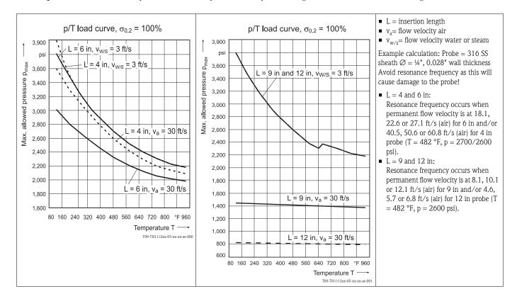
Max. allowable process pressure (PSIG) for instrumentation with one time adjustable compression fittings.
