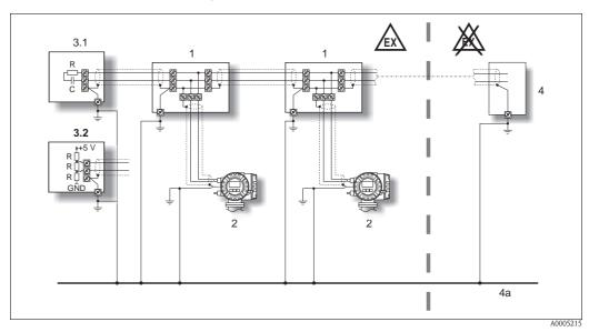
Fig. 5: Example for connecting potential equalization lines
