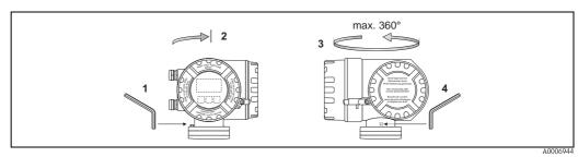
Fig. 1: Turning the transmitter housing
