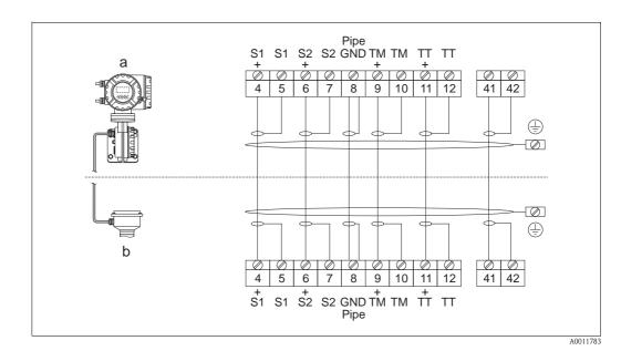
*Fig. 6: Connection of remote version connecting cable*
