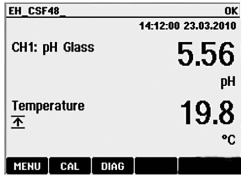
Fig. 5: Example of measuring menus
