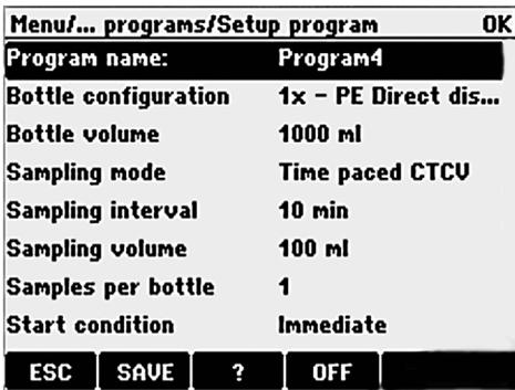
Fig. 4: Example of program setup
