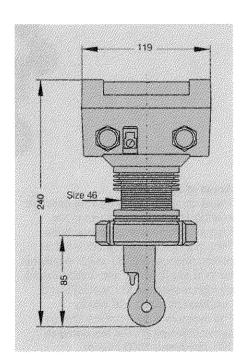
The sensor, injection-moulded from highly chemically, mechanically and thermally resistant PEEK (polyether ether ketone), does not have joints or crevices and is therefore biologically safe.
