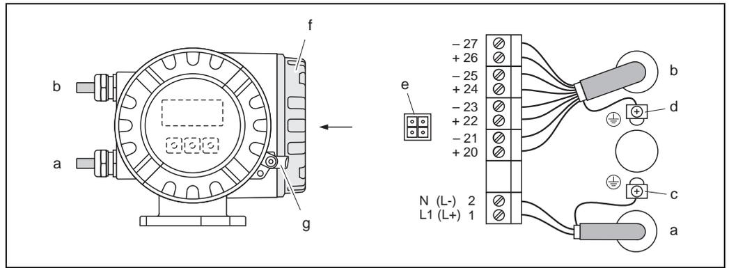
Fig. 20: Connecting the transmitter (aluminum field housing); cable cross-section: max. 2.5 mm<sup>2</sup>
