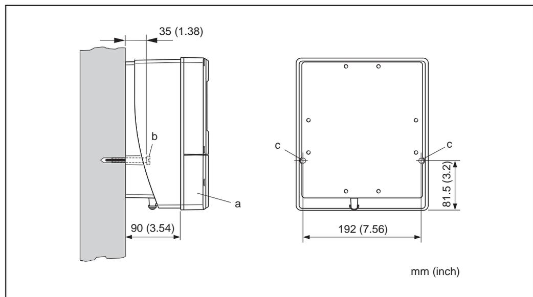
Fig. 15: Mounted directly on the wall
