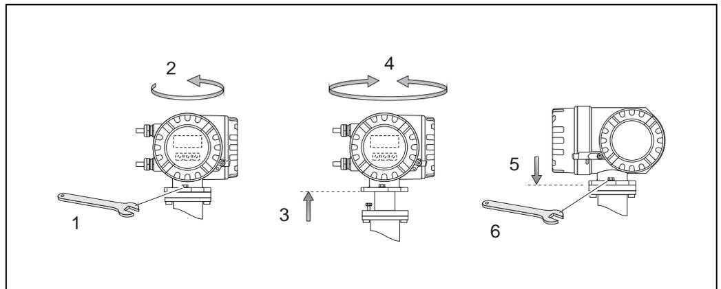
Fig. 13: Turning the transmitter housing (aluminum field housing)
