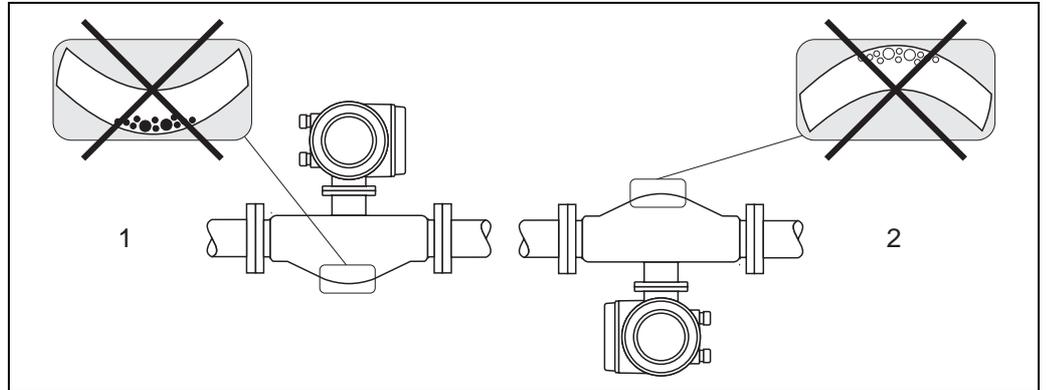
Fig. 7: Horizontal installation of sensors with curved measuring tube.
