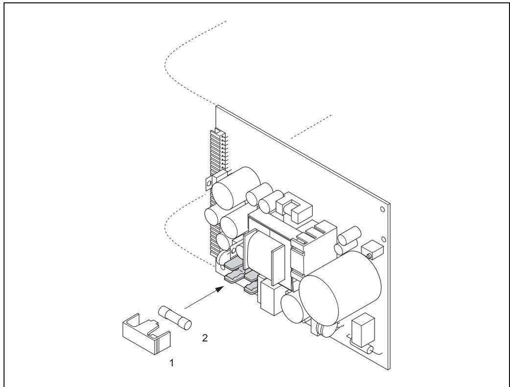
Fig. 36: Replacing the device fuse on the power unit board
