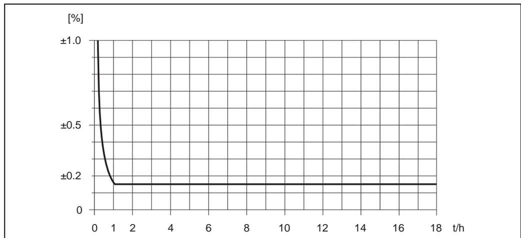
Fig. 40: Max. measured error in % o.r. (example: Promass H, DN 25)
