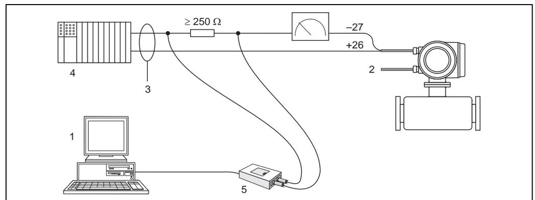
Fig. 24: Electrical connection of a PC with operating software
