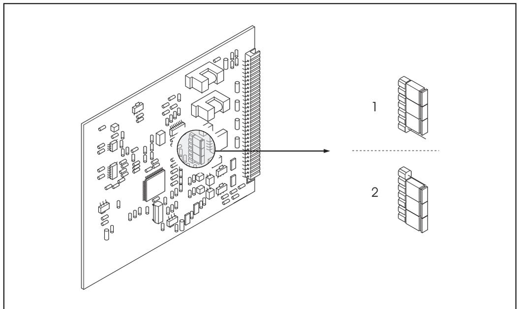
Fig. 30: Configuring the current output (I/O board)
