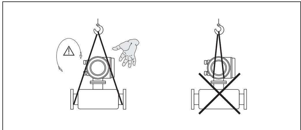
Fig. 4: Instructions for transporting sensors with  $> \text{DN } 40$  ( $1 \frac{1}{2}$  ")
