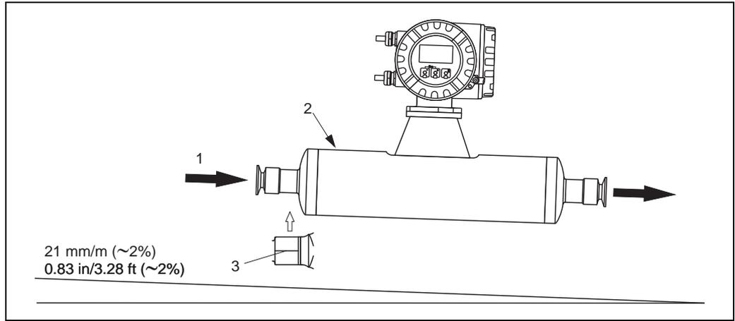
Fig. 9: Promass I: When lines are pitched in a specific direction and at a specific slope: as per hygienic guidelines (21 mm/m or approximately 2%). Gravity can be used to achieve complete drainability.
