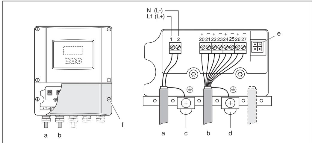
Fig. 22: Connecting the transmitter (wall-mount housing); cable cross-section: max. 2.5 mm<sup>2</sup>
