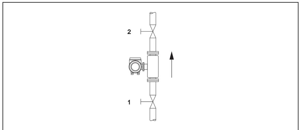
Fig. 32: Zero point adjustment and shutoff valves
