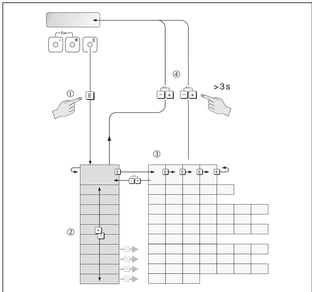
Fig. 27: Selecting functions and configuring parameters (function matrix)
