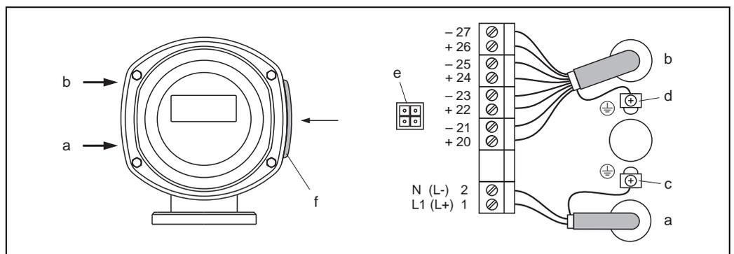
Fig. 21: Connecting the transmitter (stainless steel field housing); cable cross-section: max. 2.5 mm<sup>2</sup>
