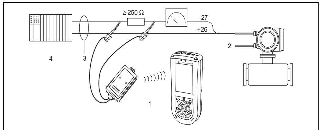
Fig. 23: Electrical connection of HART handheld terminal
