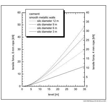
Since the tensile forces are also heavily dependent on the viscosity of the product, a higher safety factor is necessary for highly viscous products and if there is a risk of cornice buildup. In critical cases it is better to use a 6 mm rope instead of a 4 mm one.
