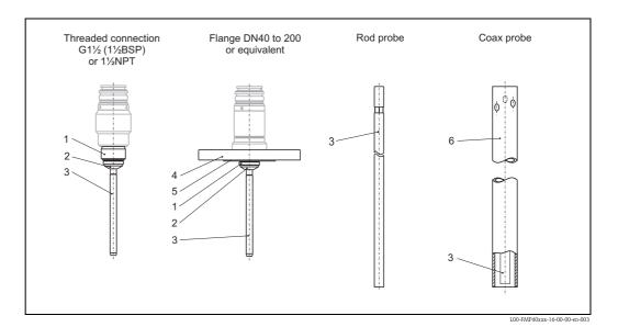
Pos. Part Material 2.4602 Adapter 2 Insulation sleeve TFM1600 3 Rod probe 2.4602 4 Flange 316L (1.4404 / 1.4435) 5 2.4602 Flange plating 2.4602 Coax probe Spacer PFA
