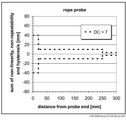
If for rope probes the DC value is less than 7, then measurement is not possible in the area of the straining weight (0 to 250 mm from end of probe; lower blocking distance).
