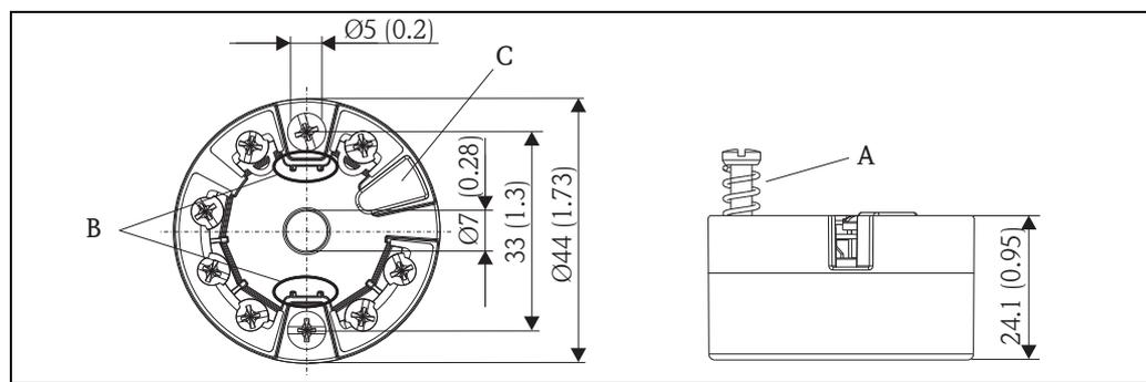
Fig. 16: Model with screw terminals
