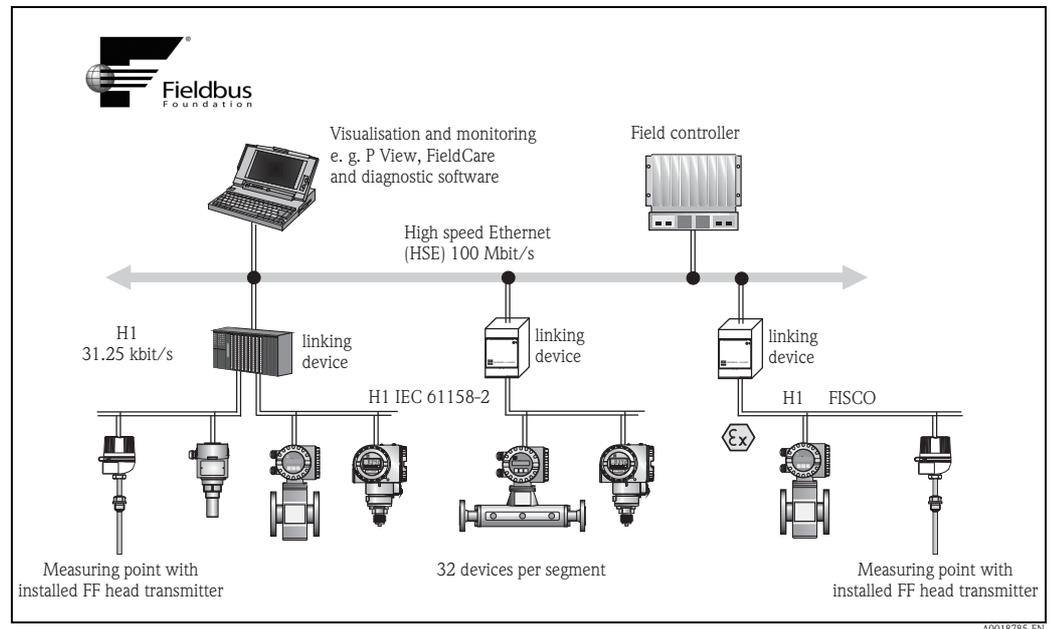
Fig. 12: System integration via FOUNDATION Fieldbus™
