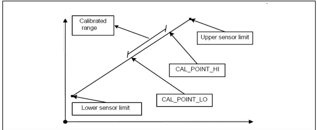
Fig. 3: Linear scaling of temperature-linear curve.
