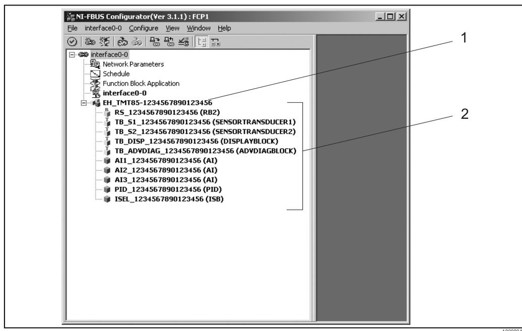
Fig. 14: Screen display in the configuration program "NI-FBUS Configurator" (National Instruments) after the connection has been established
