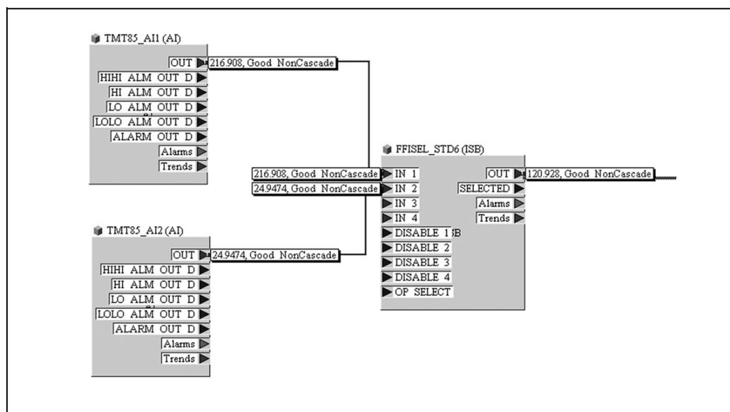
Fig. 15: Connecting function blocks with the aid of the “NI-FBUS Configurator” Example: Averaging (output OUT in the Input Selector Block) of two temperature inputs (OUT in the Analog Input Blocks 1 and 2).
