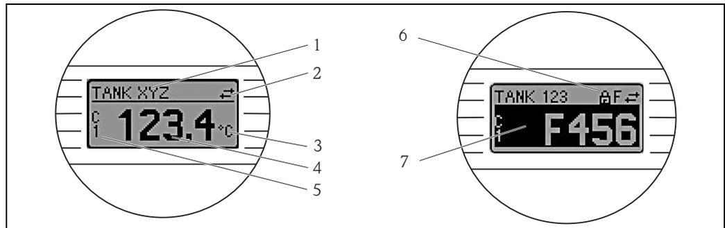
Fig. 11: Optional LC display of the head transmitter
