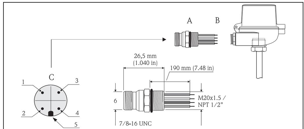
Fig. 9: Connectors for connecting to the FOUNDATION Fieldbus™
