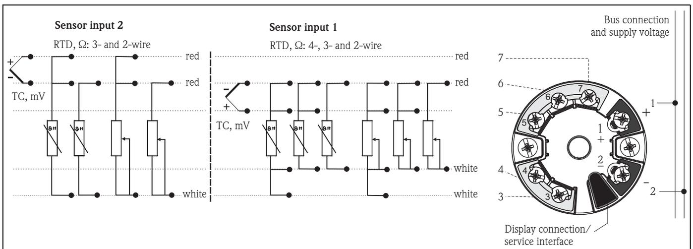
Fig. 5: Wiring the head transmitter
