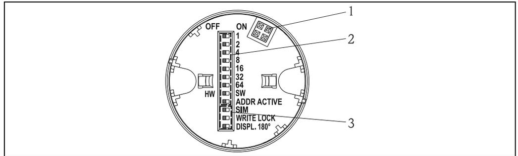
Fig. 13: Hardware settings via DIP switches
