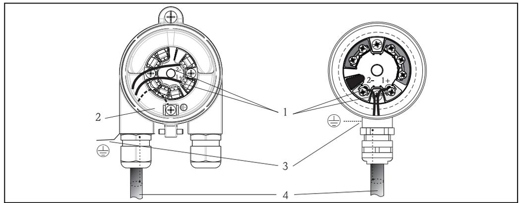
Fig. 8: Connection to the FOUNDATION Fieldbus™ fieldbus cable - installed in the field housing on the left, and in the terminal head on the right
