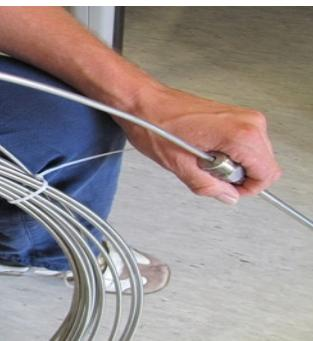
Please do not roll out the measurement insert on the ground (see picture left) or draw a spiral on the role (see picture right), since then this can not be inserted into the thermowell.
