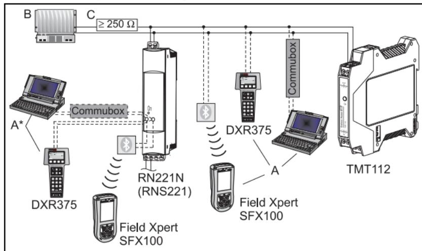
A = Connection HART® communication directly to the transmitter
