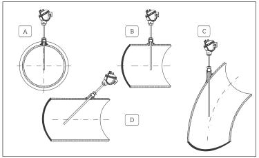
A, B: In pipes of a small section the axis line of the duct must be reached and if possible slightly exceeded by the tip of the probe.
