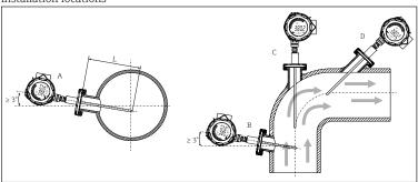
A - B: In pipes with a small cross section the sensor tip should reach or extend slightly past the center line of the pipe (=L). Installation with minimal 3° inclination because of self draining.
