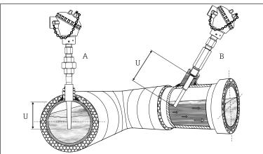
*Examples of pipe installation. In pipes of a small section the axis line of the duct must be reached and if possible slightly exceeded by the tip of the probe (=U).*
