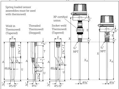
\*For thermowells with ½" NPT - 1" Process thread length and ¾" Hex length dimensions are reversed.
