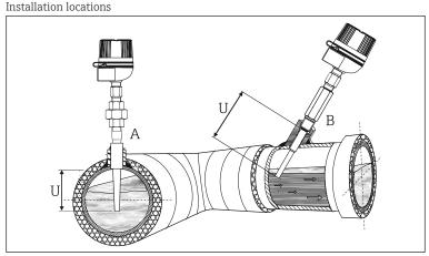
Examples of pipe installation. In pipes of a small section the axis line of the duct must be reached and if possible slightly exceeded by the tip of the probe (=U).
