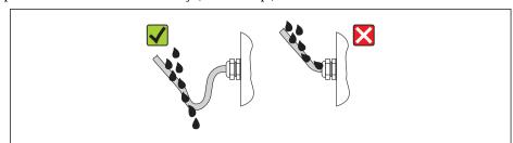
5. Insert dummy plugs into unused cable entries.
