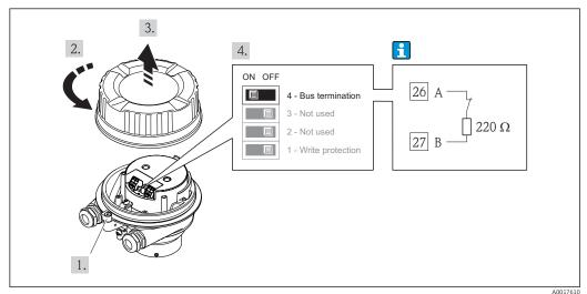
$\blacksquare$  14 Terminating resistor can be enabled via DIP switch on the main electronics module
