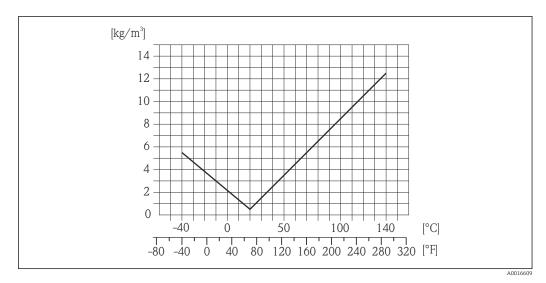
$\blacksquare$  17 Field density calibration, for example at +20 °C (+68 °F)
