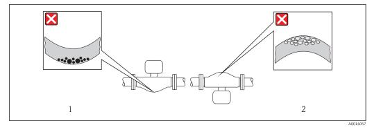
$\blacksquare$  6 Orientation of sensor with curved measuring tube
