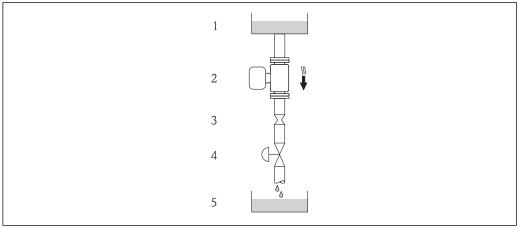
**₽** 5 Installation in a down pipe (e.g. for batching applications)
