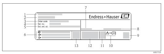
■ 2 Example of a transmitter nameplate
