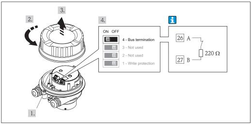
$\blacksquare$  13 Terminating resistor can be enabled via DIP switch on the main electronics module
