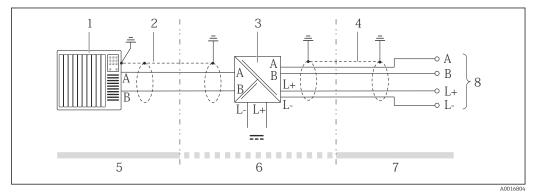
Electrical connection between the transmitter and Safety Barrier Promass 100
