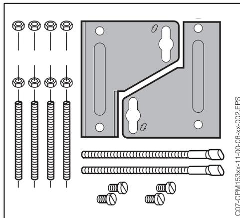
Fig. 3: Mounting kit Mycom S CPM 153
