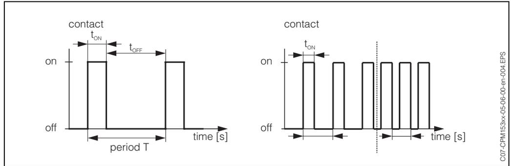
Fig. 18: left: pulse-width modulation (PWM)
