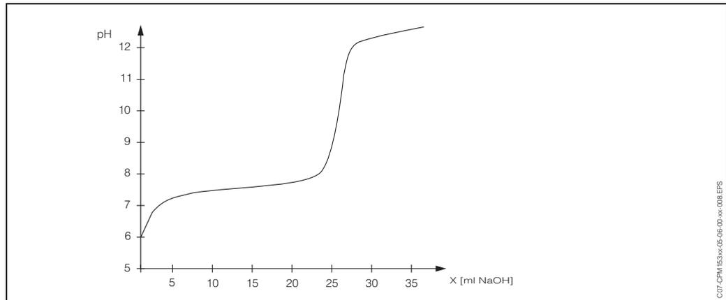
Fig. 21: Schematic titration curve of a weak acid with a strong alkali.
