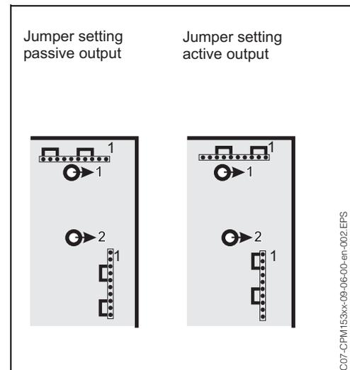
Fig. 31: Coding for passive or active current outputs
