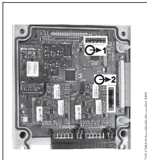
Fig. 30: Coding for active current outputs
