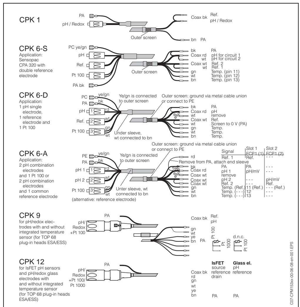
Fig. 10: Preterminated special measuring cables to connect pH and redox electrodes.
