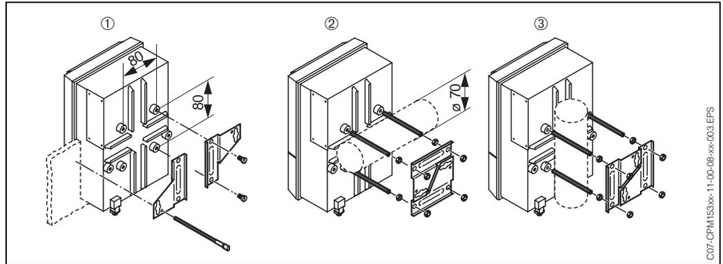
Fig. 4: Panel mounting ① and post mounting for CPM 153, horizontal ② and vertical ③
