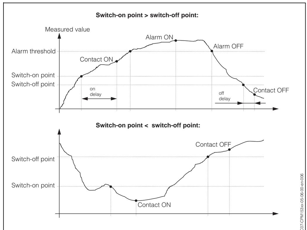
Fig. 26: Diagram of the relationship between switch-on and switch-off points and on and off delay
