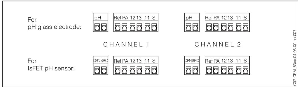
Fig. 8: Terminal assignment in the housing cover of the transmitter
