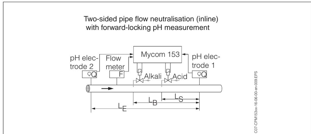
Fig. 16: Scheme of an two-sided inline process with a look-ahead pH measurement
