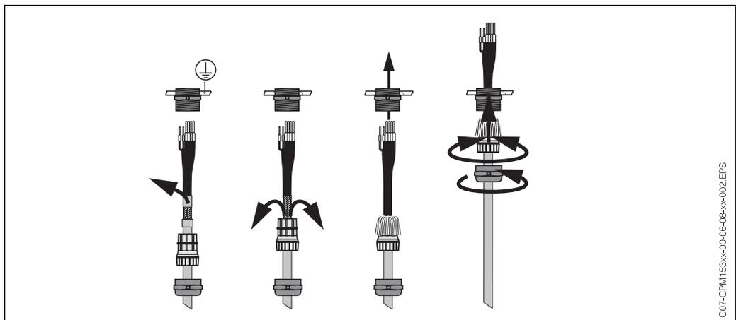
Fig. 13: Outer screen connection for CPK 1 to CPK 12 with metal cable gland. The screen contact is within the cable gland.
