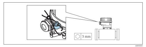
■ 1 Example of sealing with a sealing screw
