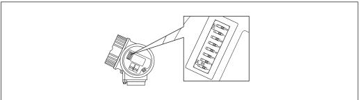
■ 13 Address switch in the connection compartment
