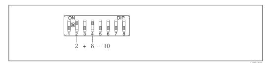
ceil 14 Example of hardware addressing; switch 8 is set to the "OFF" position; switches 1 to 7 define the address.
