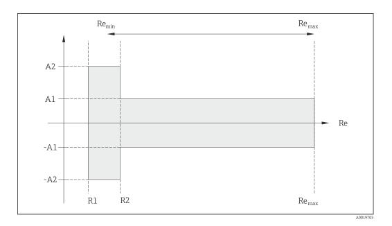
Deviation of volume flow value (absolute) from the reading Incompressible Compressible 1) Medium type Measured value deviation Re range Standard Standard R1 to R2 A2 < 10 % < 10 % R2 to  $Re_{max}$ < 0.75 % Α1 < 1.0 %
