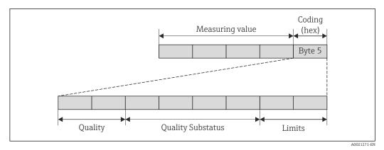
■ 32 Structure of the coding byte
