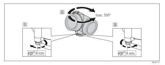
1. Release the fixing screw.
