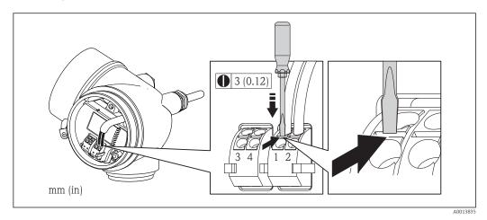
► To remove a cable from the terminal, use a flat-blade screwdriver to push the slot between the two terminal holes while simultaneously pulling the cable end out of the terminal.
