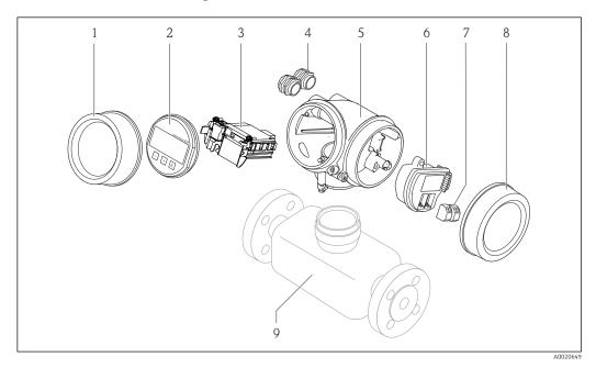
$\blacksquare 1$  Important components of a measuring device
