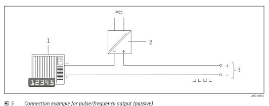
Connection example for pulse/frequency output (passive)
