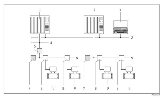
$\blacksquare$  27 Options for remote operation via FOUNDATION Fieldbus network
