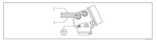
1 Cable entries for inputs/outputs
