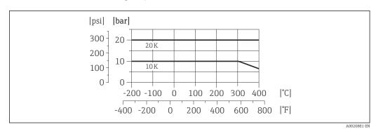
$\blacksquare$  18 Process connection material: stainless cast steel, multiple certifications, 1.4408 (CF3M)
