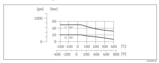
■ 17 Process connection material: stainless cast steel, multiple certifications, 1.4408 (CF3M)
