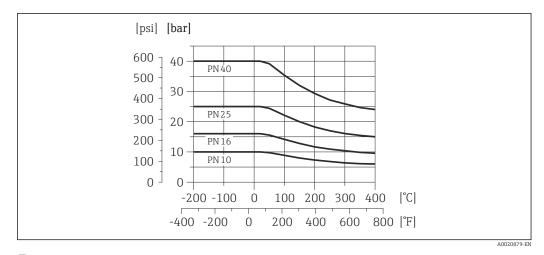
■ 16 Process connection material: stainless cast steel, multiple certifications, 1.4408 (CF3M)
