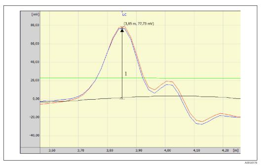
1 Absolute echo amplitude in the envelope curve as measured from the 0mV line
